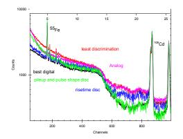
Figure 3. Manganese and silver K x-rays spectra superimposed on 133Ba nuclear and Compton background. The shape of the Compton profile depends on the signal processing approach
