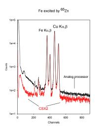
Figure 1. An Fe sample is irradiated with Cu K radiation from a 65Zn source in transmission geometry. The background is substantially reduced using the CSX2 or CSX3 by noise discrimination and risetime discrimination. The manufacturers analog processor (--), and the Cambridge Scientific CSX2 digital processor (---)
